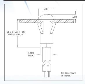
Mounting: Will snap-fit into  $\emptyset$ .500/.505 hole in panels .020/.100 thick. Push-on speednut SN0461 also available.
